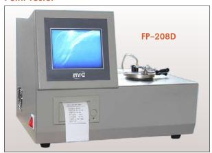
This instrument is designed and made as per GB/T 5208–2008 Determination of flash point – Rapid equilibrium closed cup method. It can meet the requirements of rapid determination for closed
